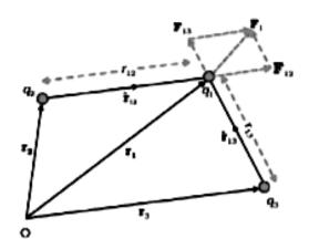
The force on one charge, say q1, due to two other charges q2, q3 can therefore be obtained by performing a vector addition of the forces due to each one of these charges. Thus, if the force on q1 due to q2 is denoted by F12, F12 is given by following Eqn. even though other charges are present. In the same way, the force on q1 due to q3, denoted by F13.
